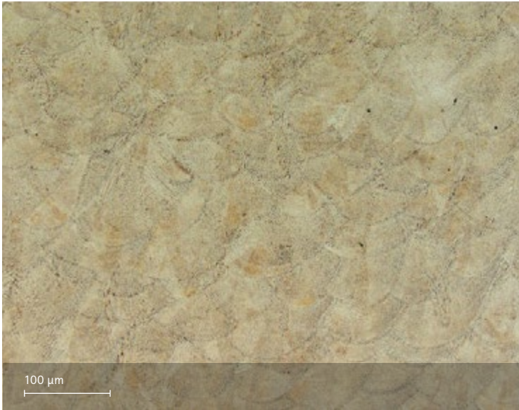
As manufactured microstructure. Etchant: Kalling's II
